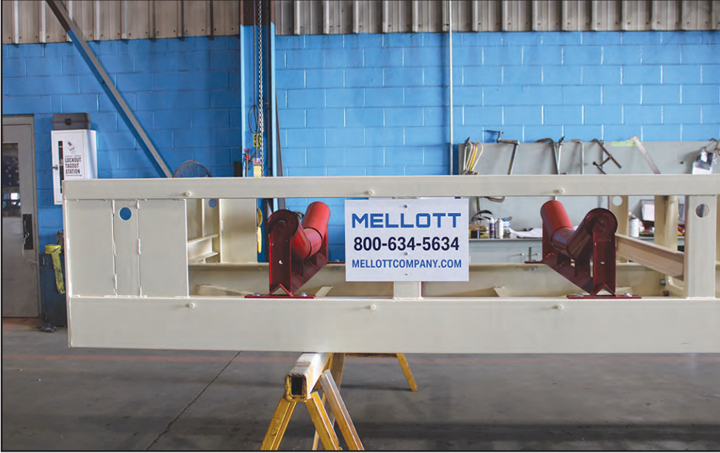
A finished component piece – shot blasted and painted – waits to be loaded for delivery.
